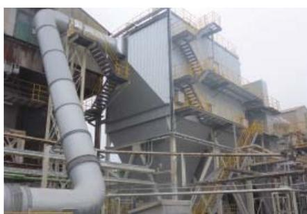
Electrostatic precipitator (Ube Material Industries, Ltd.)
