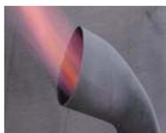
Model exhaust pipe made using a TYRANNO FIBER composite
