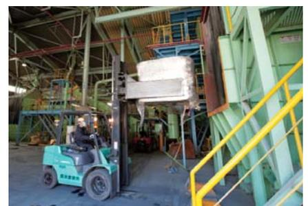
Inserting waste plastic into treatment facility
