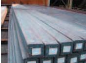
Billets (steel ingots for rolling)
